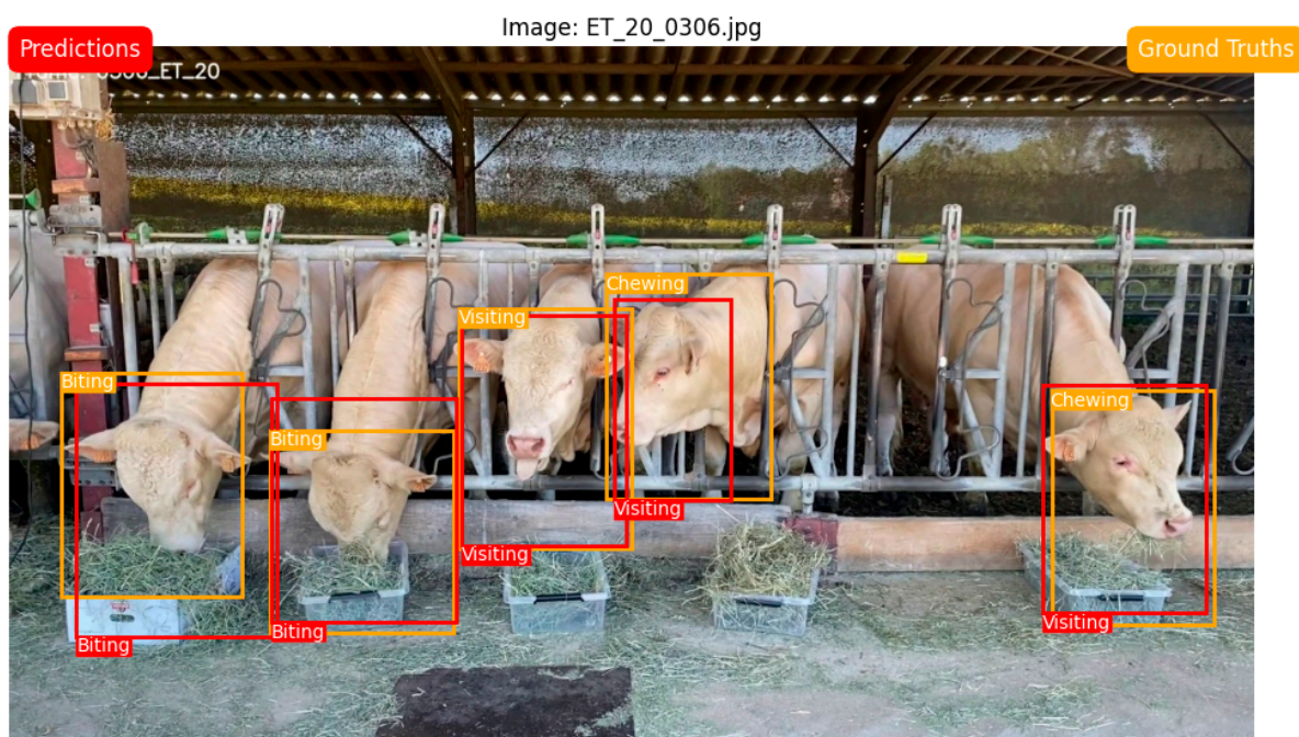
Figure 6. Capture of a frame showing the YOLOv8 prediction of feeding activities of individual beef cattle animals.
