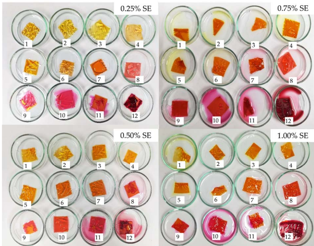
Figure 1. pH sensitivity of gelatin films incorporated with sappan heartwood extract at different concentrations. SE: sappan heartwood extract. The number donated the pH level.
