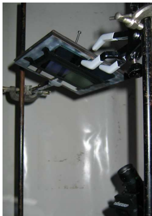
Fig. 1. a) The catadioptric viewer composed of a CCD monochrome camera with 2 mirrors placed above the camera. An interferential filter is fixed on each mirror. b) Optical model of the viewer system considering only one mirror (M1).
