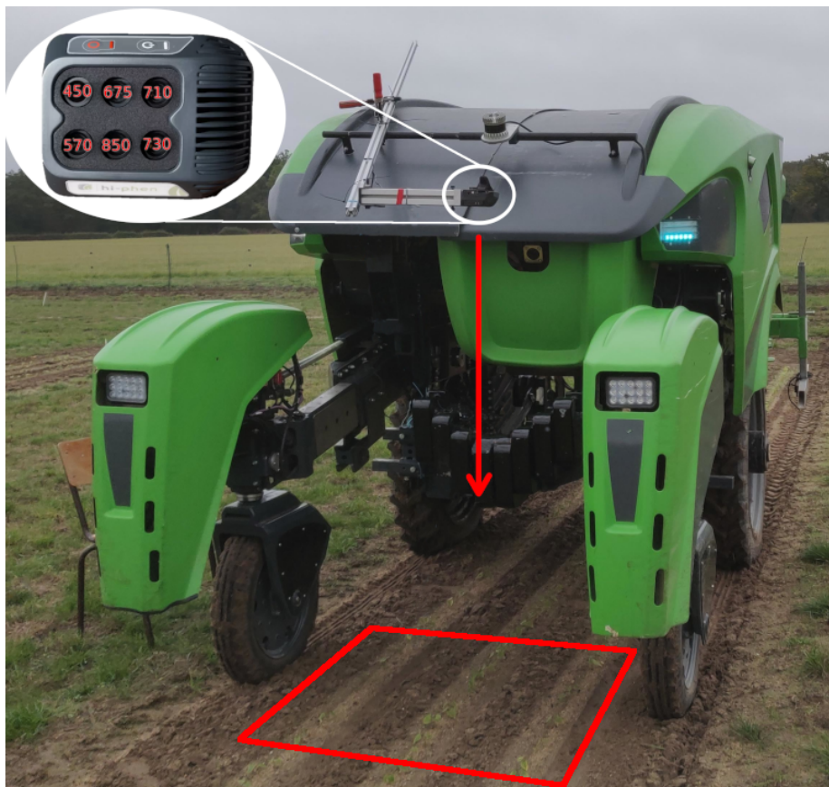
Figure 2: The experimental set-up : the multispectral camera and the robotic platform
