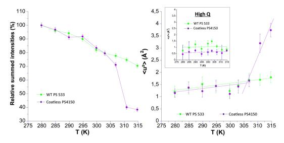
**Figure 4.** Temperature dependence of the relative summed intensities (left sight) and MSDs (right side) of spores produced on SPZ agar medium in  $D_2O$  suspension: WT PS533 (green) and Coatless PS4150 (purple) spores. MSDs are extracted at low Q, and insert show the MSDs extracted at high Q where germination has no effect. The straight lines on the right side are linear fits to extract the effective force constants (see Table 3).
