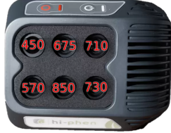
Figure 1: Disposition of each band on the Airphen multi-sensors camera
